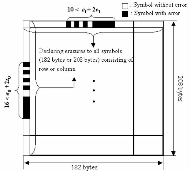
Fig. 2. The incorrect erasure declaration under the conventional decoding rule of RS-PC.
