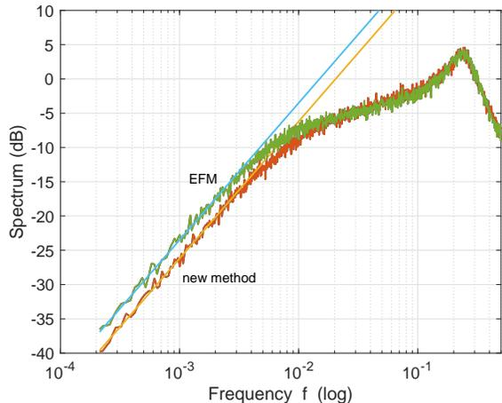
Fig. 2. Spectrum of classic EFM and the new method (dB) versus relative frequency  $f$  (log axis).
