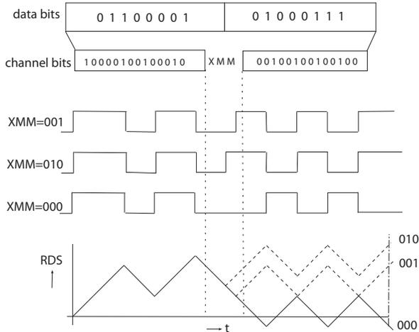
Fig. 1. Strategy for minimizing the running digital sum (RDS) in EFM. Two 8-bit user words are translated into 14-bit codewords using a look-up table. The 14-bit codewords, in turn, are cascaded, ‘merged’, using a 3-bit merging word in such a way that the runlength conditions continue to be satisfied for the cascaded sequence.
