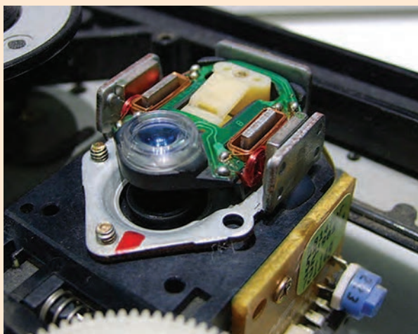
A typical laser optical assembly. Note that all six focusing and tracking coils can be seen. While tracking of the laser system could introduce random bit errors, the main challenge was that of long burst errors due to scratches or dust. (Photo courtesy of Wikipedia.)
